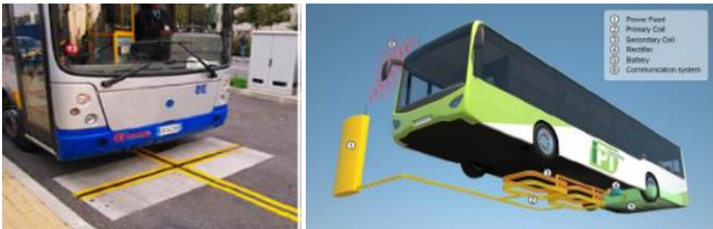
Figure 21: IPT Charge System
