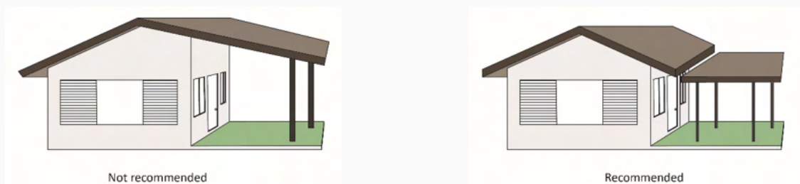
FIGURE 9 Recommended separation of veranda shelter from main building
