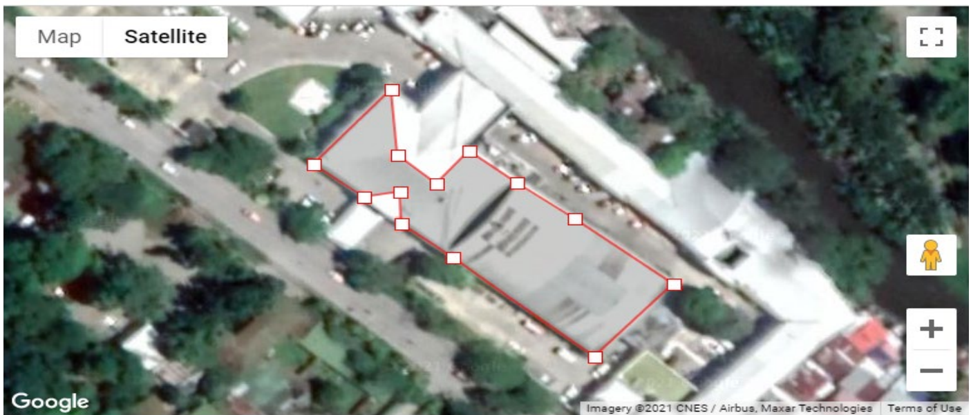
Figure 5. The customized rooftop area layout for 300-kW solar PV system of PGOM Main Building using the PVWatts Calculator. Further detailed designs will be needed for both layouts during the full feasibility studies. These will involve structural analysis.
