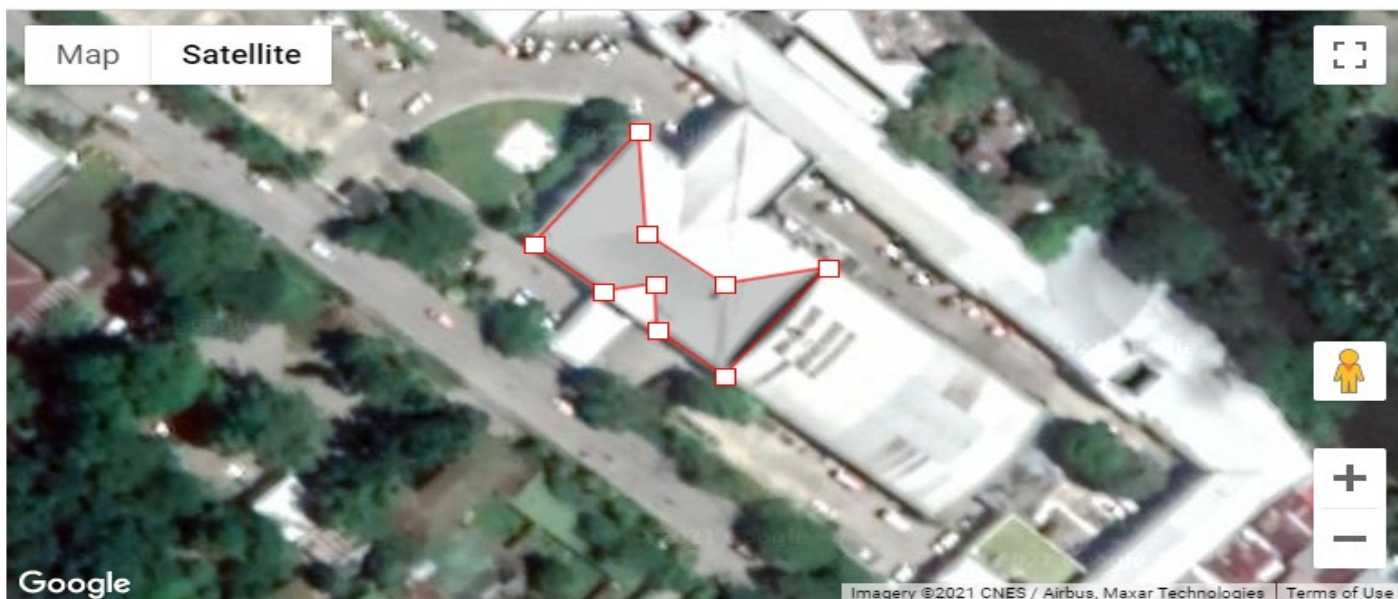
Figure 4. The customized rooftop area layout for 100-kW solar PV system of PGOM Main Building using the PVWatts Calculator
