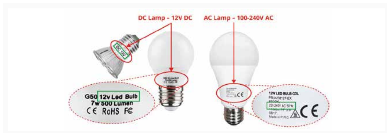
FIGURE 2.4 Information on DC and AC power supply for LED lamps
